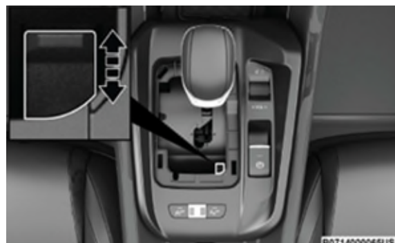
Gear Selector Override Access Location
